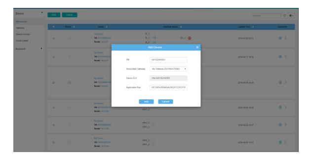
4 Click to configure the UC11-N1 from Ursalink cloud and add channel for the Modbus. **Note:** Channel name should be as same as the one set in UC11-N1.
