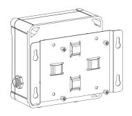
B. Mount the mounting bracket horizontally to the wall by fixing the screws into the wall plugs.
