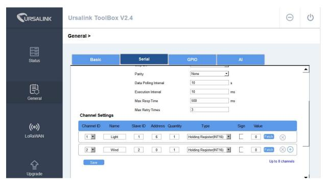
In this Quick Start Guide, UC11-N1 connects with two equipment (light sensor and wind speed sensor), both sensors use Modbus RS485.
